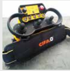
REMOTE CONTROL Comfortable and lightweight for the boom control and for the management of the main functions of the machine.
