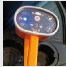
CABIN CONTROLS Electro-hydraulic controls placed in the cabin to adjust all main functions of the truck mixer pump and the motors.
