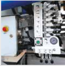
BOOM PROPORTIONAL DISTRIBUTOR Ergonomic hydraulic controls for boom and stabilization system.
