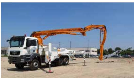
All outriggers are designed to stabilize the machine in the right way in extraordinary tight spaces.
