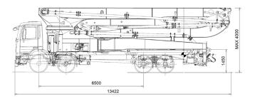
Dimensions varying according to truck assembly
